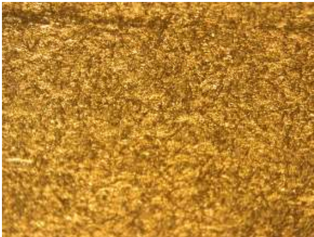
Fig 4.7 Microstructure of test specimen (96% Al, 4% SiC)
