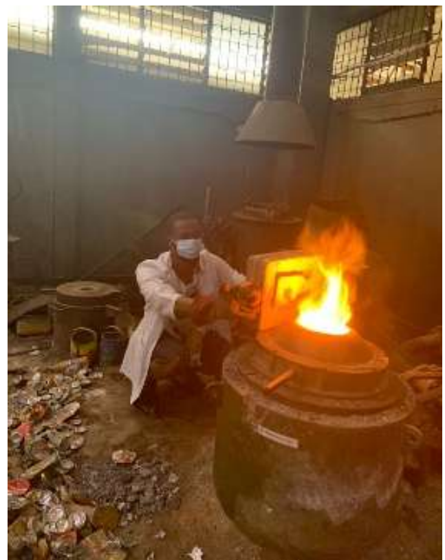
FIG 3.2 Heating of the Aluminum in a furnace
