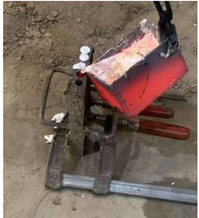
FIG 3.4 Pouring of the composite in a former
