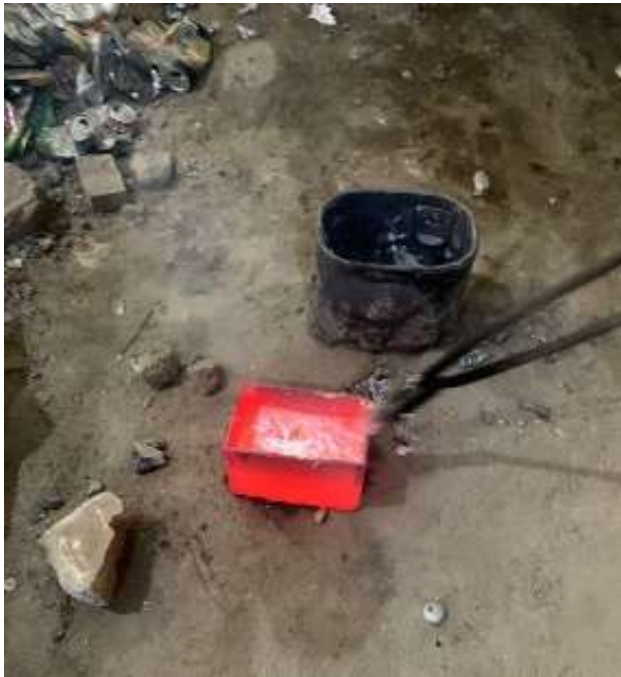
FIG 3.3 Melted Aluminum alloy with silicon carbide powder (stirred)
