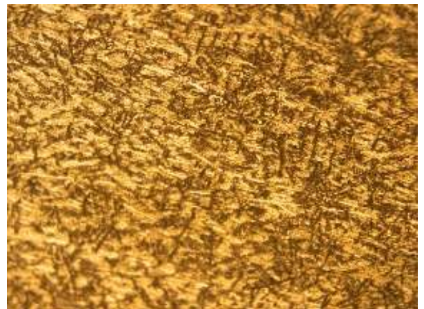
Fig 4.8 Microstructure of test specimen (94% Al, 6% SiC)
