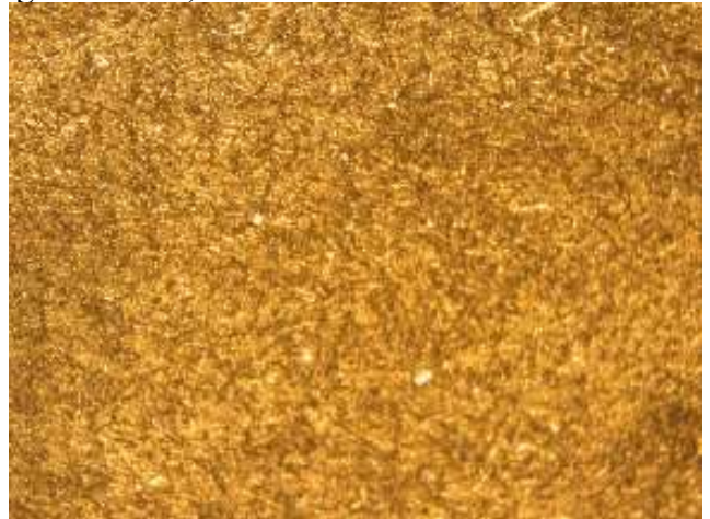
Fig 4.6 Microstructure of test specimen (98% Al, 2% SiC)
