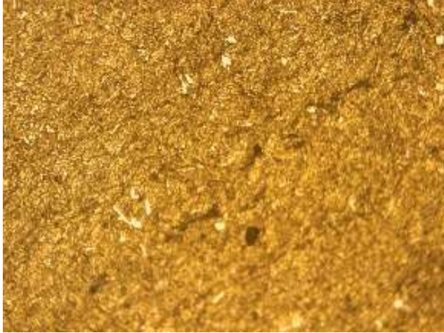
Fig 4.5 Microstructure of control (100% Al)
