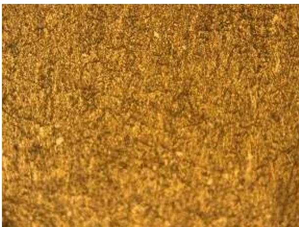
Fig 4.7 Microstructure of test specimen (96% Al, 4% SiC)
