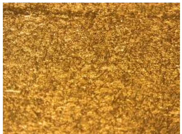
Fig 4.8 Microstructure of test specimen (94% Al, 6% SiC)
