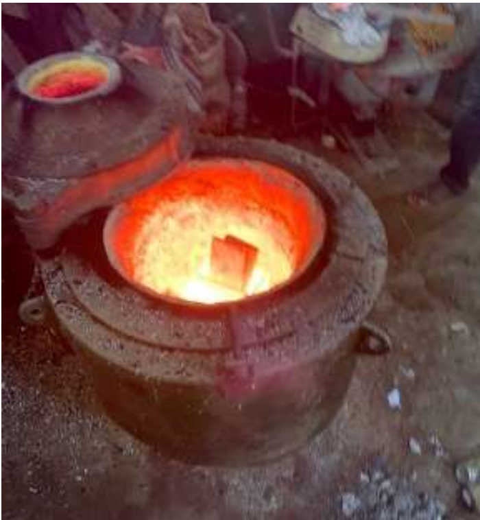
FIG 3.1 Melting of the Aluminum in a furnace
